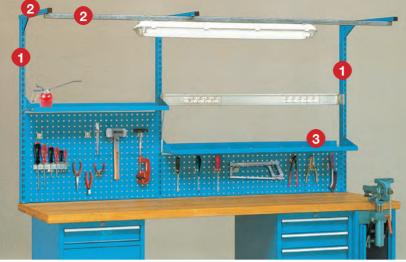
**Vertical rods** - In bi-slotted steel profile Max load capacity 50 kg
